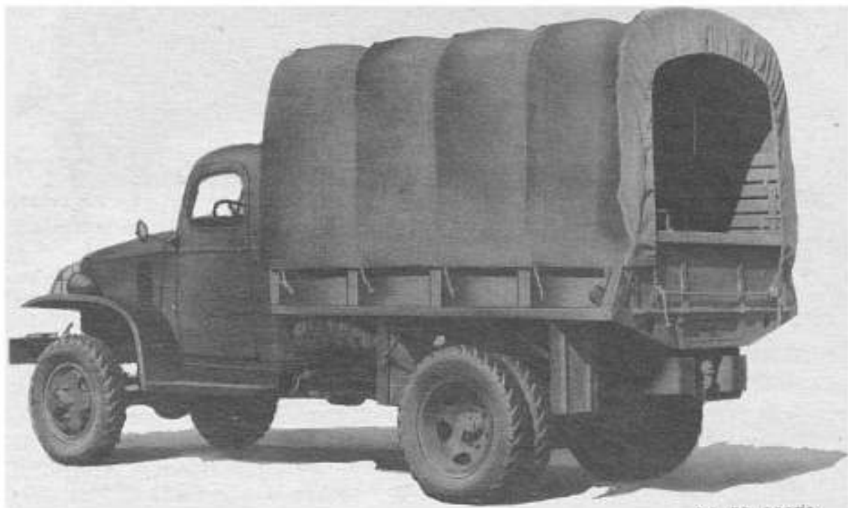
Figure 4—Chevrolet 1 1/2-Ton, 4 x 4 Truck Model G-7107—Cargo less Winch Model G-7117—Cargo with Winch
