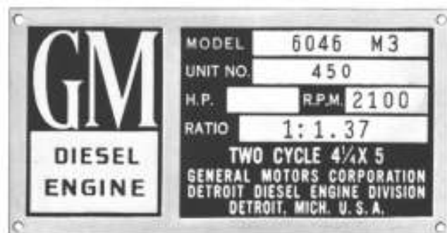
Fig. 8—Typical Unit Number Plate Used on Later (M-3A5) Power Units.
