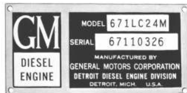
Fig. 6—Typical Serial Number Plate Used on LC Engine.
