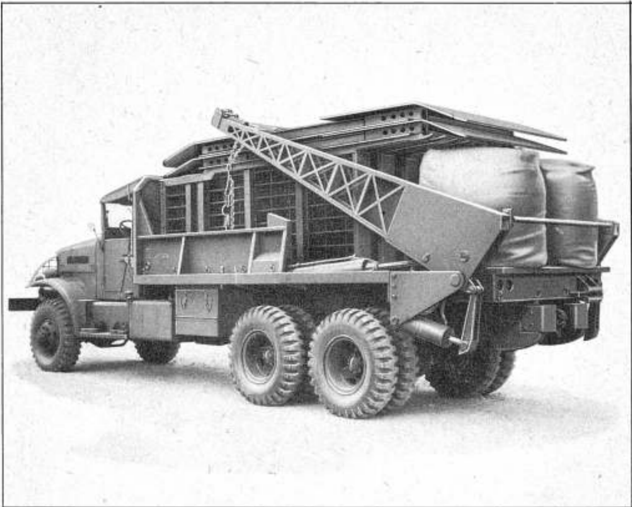
Figure 1. Hydraulic Bridge Erecting Crane with Typical Load
