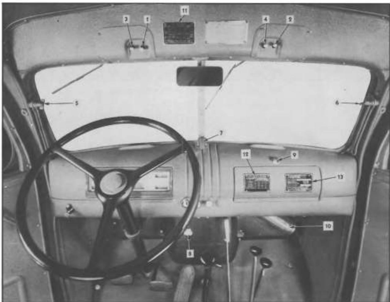
Fig. 2—Interior of cab, showing Driver Instruction plates, etc.
