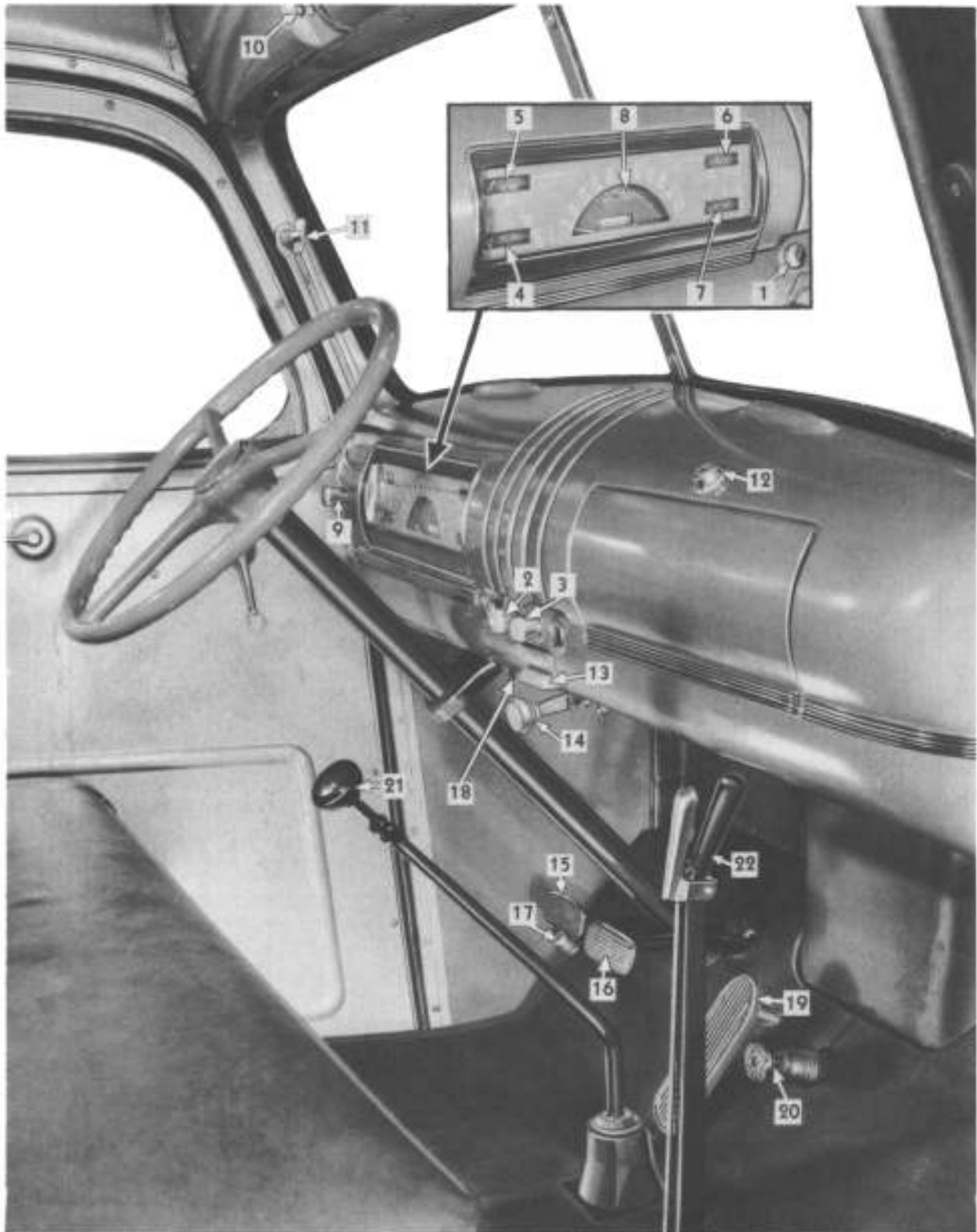
Fig. 1—Interior of Cab showing Location of Instruments and Controls
