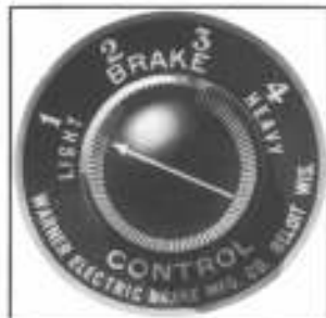
Fig. 7—Trailer Electric Brake Load Control
