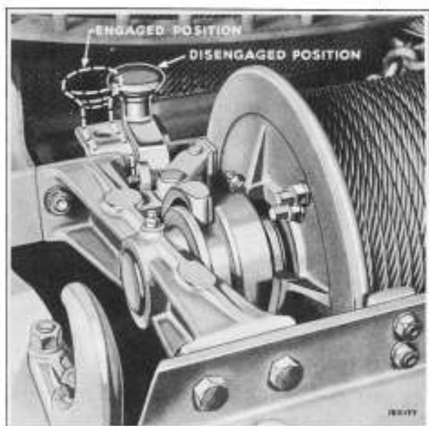
Fig. 6—Winch Clutch Shifter Fork Handle Positions
