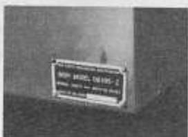
CARGO BODY —Model number plate on lower L. H. front corner of body.
