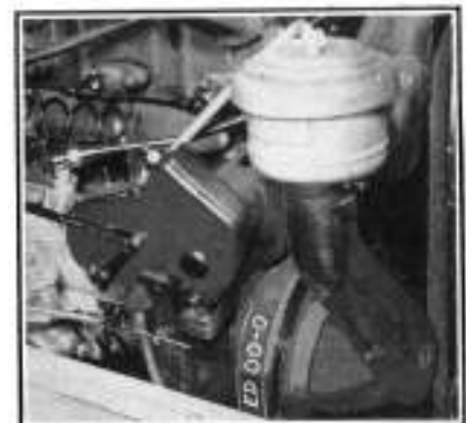
Engine Serial Number stamped on right side of timing gear housing
