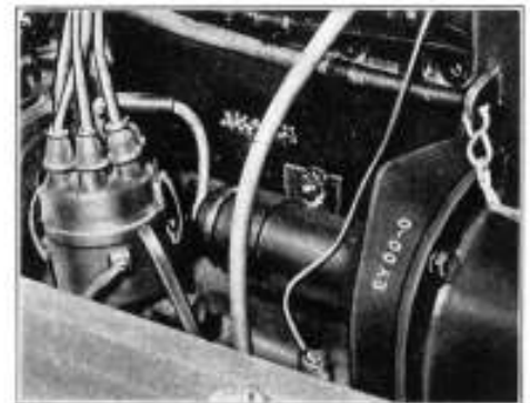
Engine Serial Number stamped on right side of timing gear housing
