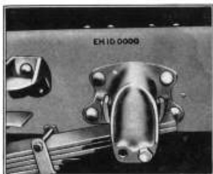
Chassis Serial Number stamped on rear end of left frame side member
