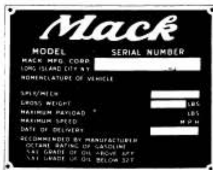
Chassis Name Plate located on instrument panel
