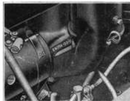
Engine Serial Number stamped on left side of cylinder block
