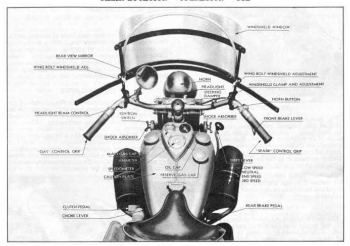
While the above illustration is taken of a Model 640-B, all controls are identical to the Model 741-B with the exception that the Model 741 the shift is located at the rear of the tank.
